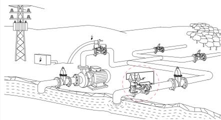
RAF 88 is located next to a booster pump to protect the supply line downstream of the pump from water hammer damages.
